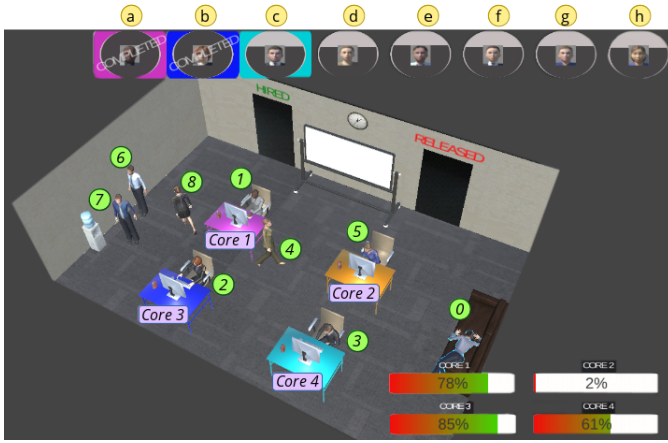
Fig. 6. Screenshot of ParallelAR executing (real-world background on mobile screen is cropped out), after combining the Fully Parallel and Identical (Coarse-grained) flashcards. With eight tasks (numbered a to h ) assigned to eight threads (numbered 1 to 8 ) and only four cores, some context switching occurs. The main thread (numbered 0 ) is sleeping (on the couch).
